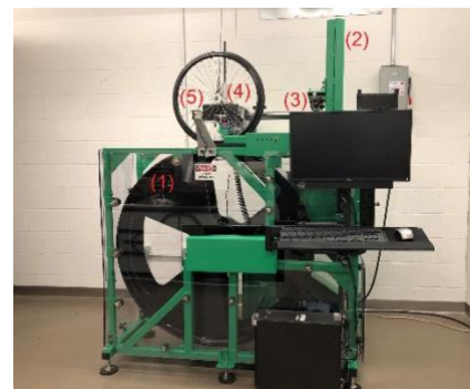
Figure 2: Drum based rolling resistance testing machine. (1) Drum, (2) Upper Frame, (3) Arm, (4) Truck, (5) Load Cell
